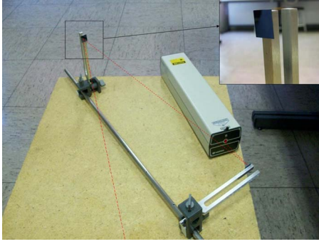
Fig. 1. Experimental setup used to produce Lissajous figures using two tuning forks. After being reflected by the two mirrors, the laser beam is projected onto a screen located 2–3 m from the table.
