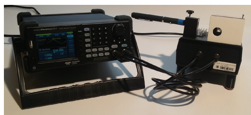
Figure 2. Setup of galvo mirrors and two-channel waveform generator.
