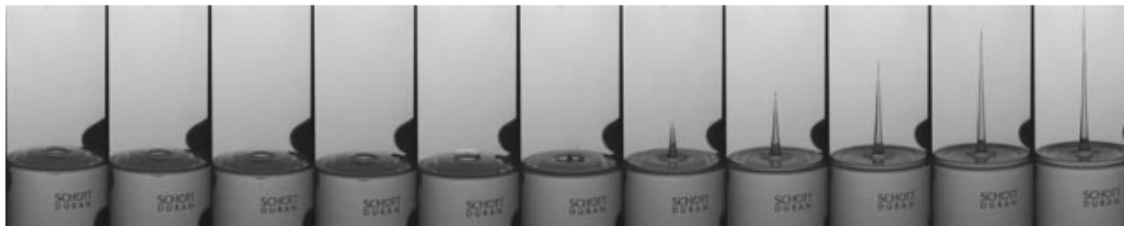
FIGURE 3. A liquid with a free surface is falling as a whole under gravity. A bubble at the free surface gives rise to a strong jet after impact. The interval separating each snapshot of this sequence is 1 ms.
