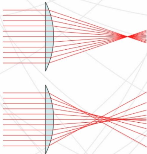
Light rays that strike a spherical surface off-centre are refracted or reflected more or less than those that strike close to the centre.
