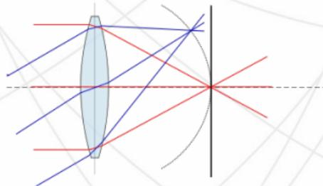
Flat object normal to the optical axis cannot be brought into focus on a flat image plane.
